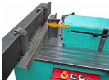
101 T- / L- / U- / H-Profile richten Profile straightening
