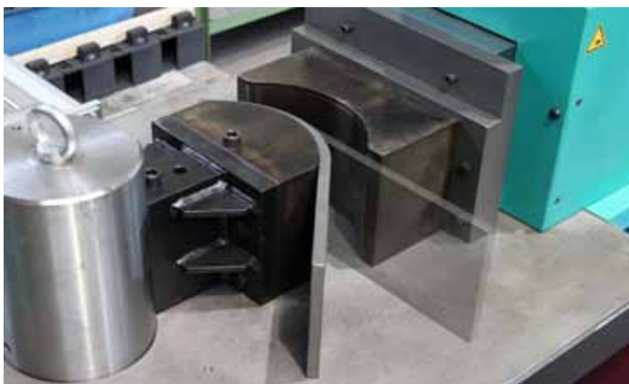
171 Pressbiegen / Formbiegen Press bending / Form bending
