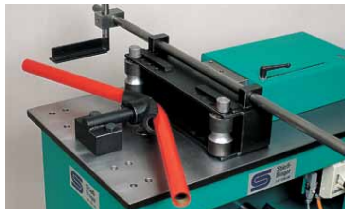
132 Gasrohrbiegen Bending of pipes
