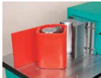
63 Biegen von geschlossenen Formen Bending of closed shapes
